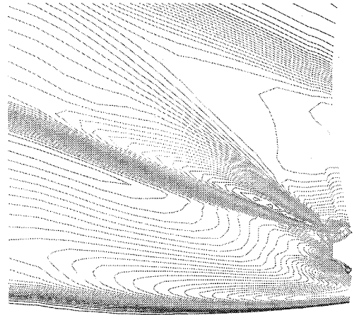
Fig. 12 Temperature contours in symmetry plane of X-33 wake at Mach 10.5 and \alpha = 26 deg.
